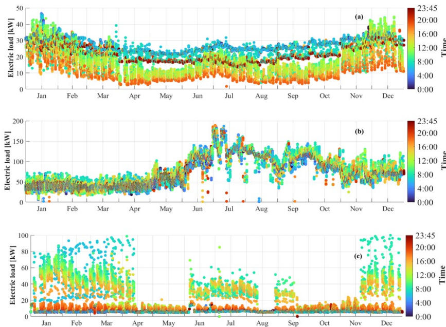
Figure 2. Electric load profiles on a quarter-hour basis of Us#1 (a), Us#2 (b) and Us#3 (c)
